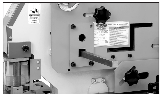
Figure 37. Example of square bar shearing setup.
